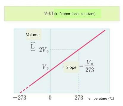
At constant pressure, the volume of a given amount of gas increases by 1/273 of its volume at  $0^{\circ}$ C for every  $1^{\circ}$ C rise in temperature, and decreases by 1/273 for every  $1^{\circ}$ C fall in temperature.
